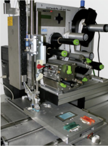
Hermes label printer with applicator from CAB
