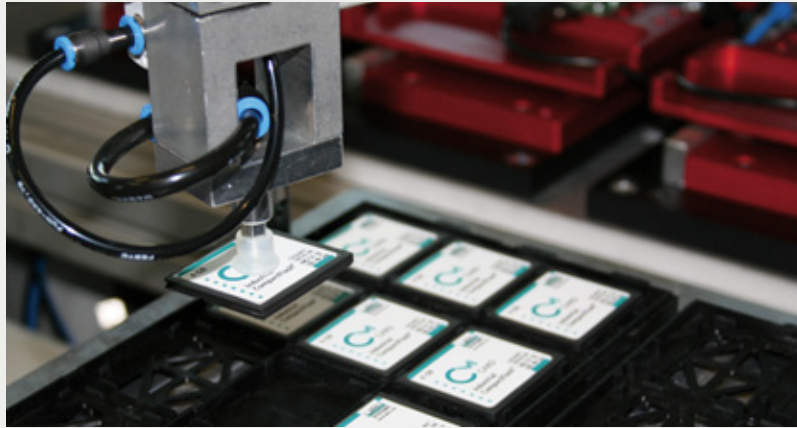
Automatic Test Equipment robots picker arm with a CodeMeter CmCard/CF
