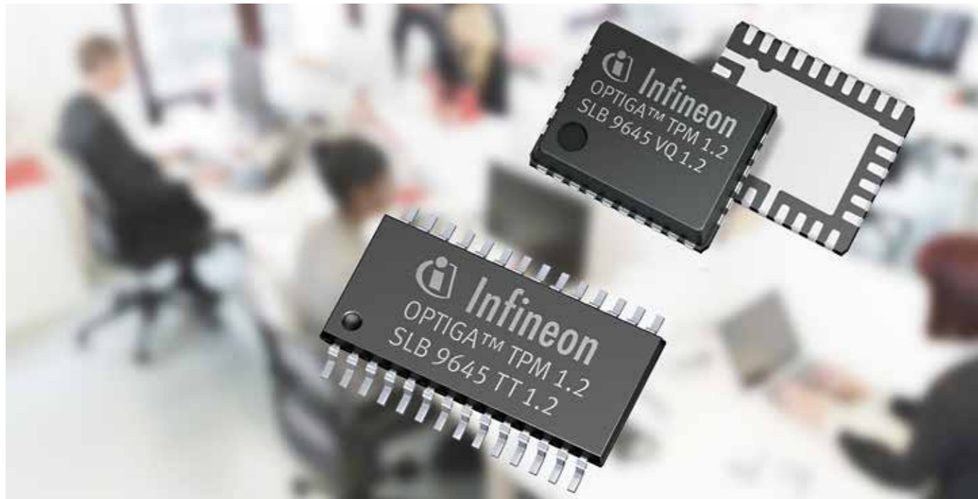
Figure 2: OPTIGA™ TPM (Trusted Platform Module) from Infineon
