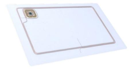
Figure 2 -Inlay Laminated Contactless Module from Infineon
