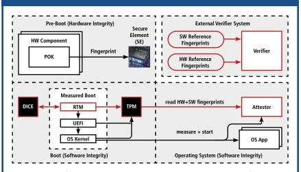
Hardware and software integrity are inextricably linked with the Trusted Platform Module (TPM) 2.0, using the TPM ecosystem (Trusted Boot, TPM 2.0 Software Stack (TSS2), and Remote Attestation). The Device Identifier Composition Engine (DICE) ensures the peripheral components' integrity on the board. Processes, protocols, and data structures are set to be standardized by the Trusted Computing Group (TCG) and the IETF.
